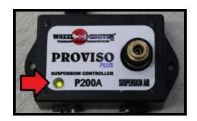
The LED can be used determine if the module is detecting any problems. The LED colour code is:
